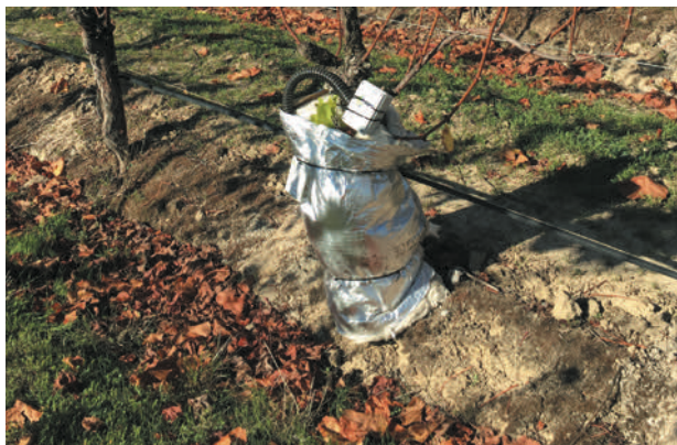
Saturas sensors measure vine water stress.
